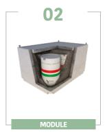
The final products are placed and cemented in special concrete modules (3 m x 2 m x 1.7 m), designed to withstand 350 years.
