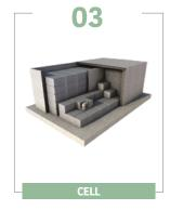
Each cell in reinforced concrete (27 m x 15.5 m x 10 m), designed to last at least 350 years, can store 240 modules.
