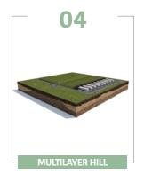
Artificial structure arranged to cover the cells. It is made of layers of different materials to prevent rainwater infiltrations, isolate the wastes from the environment and improve the visual impact of the structure.
